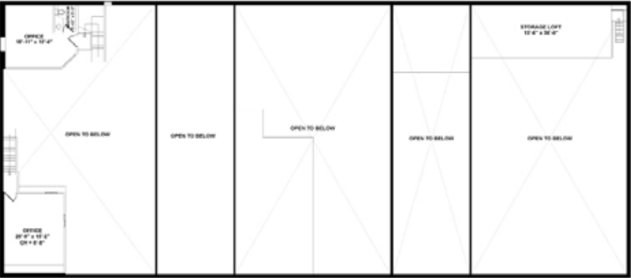
MEZZANINE FLOOR PLAN Ceiling Height = 7'-0"
